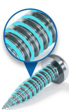
Due to the generated pull-through, the created internal thread is longer than the sheet thickness. In addition the thread pitch of QUICK FLOW® Plus is finer than the pitch of conventional sheet screws, which means that there is sufficient overlap of the formed thread flanks to create a stable joint. The QUICK FLOW® Plus thin sheet screw has a double thread. This additionally increases the surface area of the engaged thread flanks.
